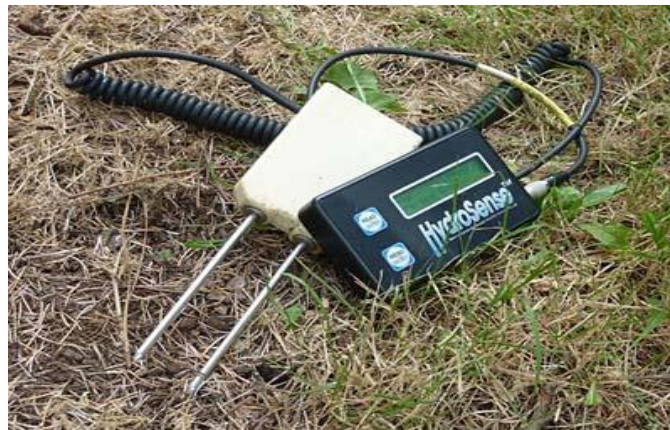
Fig. 3. Time Domain Reflectometry (Source: labmodules.soilweb.ca )
