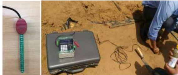
Fig. 5. A VH400 sensor; its Data logger
