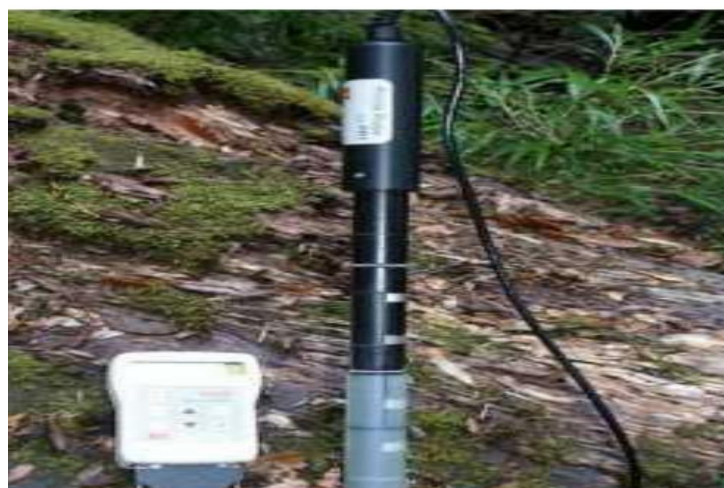
Fig 4. Frequency Domain Reflectometry (Source: www.experimental-hydrology.net )
