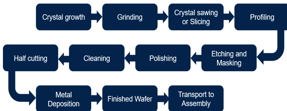
Fig. 3. Wafer fabrication flow
