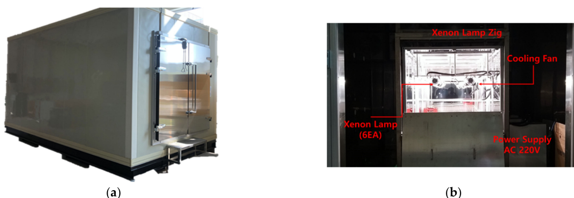
Figure 1. Photographs of the (a) exterior and (b) the interior of the PV panel experimental chamber.
