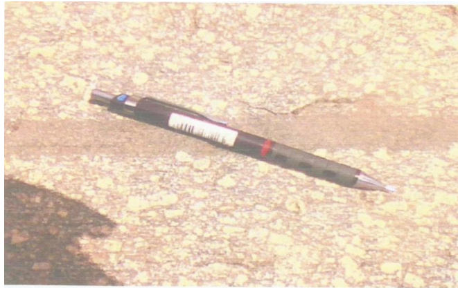
Fig. 4. Field photograph of Xenolith observed on a porphyritic granite due to incomplete obliteration of the country rock at location with the coordinates latitude 11°35' 27.2"N and longitude 007°32' 07.8"E
