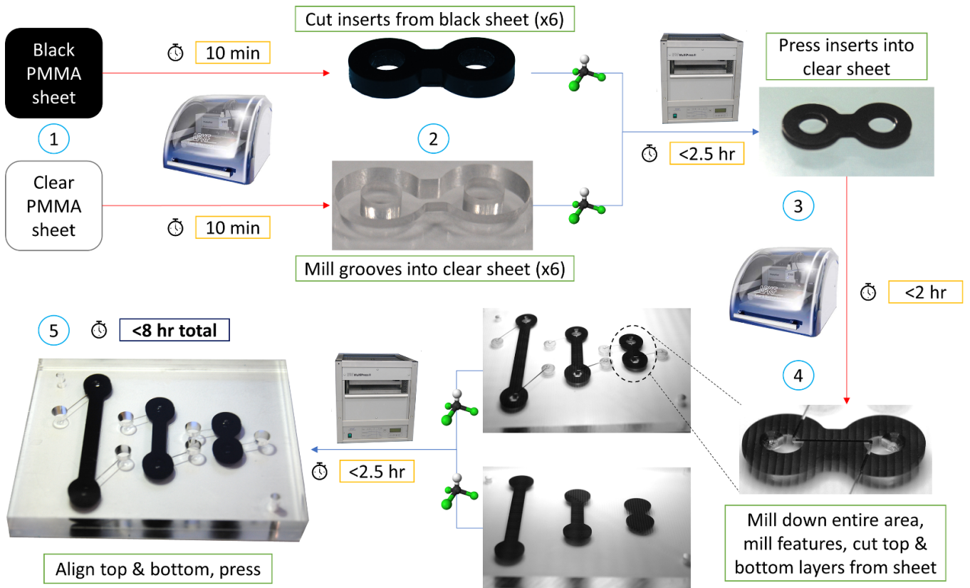
Figure 2. Fabrication process of a microfluidic chip containing three inlaid absorbance cells of varying lengths. Plastic milling occurs via an LPKF S103 Micromill and bonding through pressing chloroform-treated layers within an LPKF Multipress II. Milling times depend on the complexity and size of the design but are listed here as upper-bounds for the depicted inlay optical chip. In step 4, the vertical patterned lines are a result of milling down the area to achieve a smooth surface.
