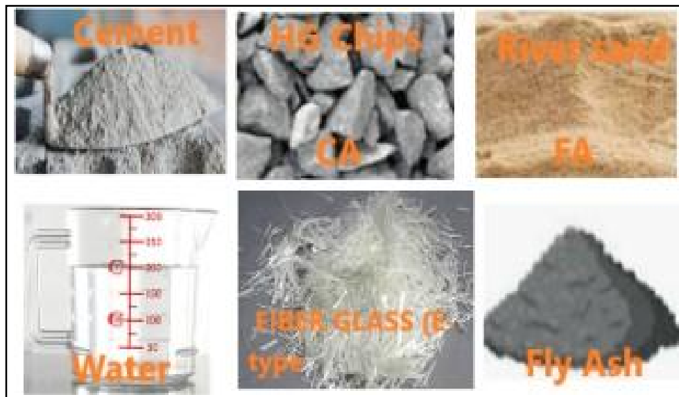
Fig. 1. Ingredients for fibre glass concrete blended by fly ash
